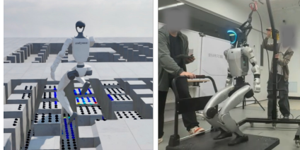
Figure 5: Robot stance without AMP. Without motion guidance, the robot constantly walk with its leg bent.
