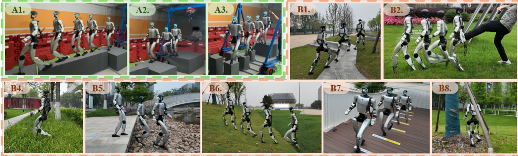
Figure 6: Real-world evaluation of TAGA from controlled indoor terrains to unstructured outdoor environments. (A) Indoor trials test limit traversal over discontinuous terrains such as platform transitions, large steps, and sparse stepping blocks. (B) Outdoor trials evaluate robustness to terrain variation, perception degradation, and external disturbances. Our results show that TAGA maintains stable locomotion across discrete foothold selection, terrain variation, and physical perturbations.
