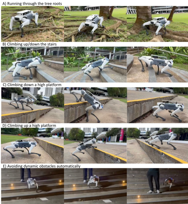
Fig. 5. Outdoor hardware experiments under low visual disturbances, including tree roots, staircases, elevated platforms, and dynamic pedestrians. With only a constant forward velocity command of [1.0, 0, 0] , the robot traversed all terrains and avoided obstacles.
